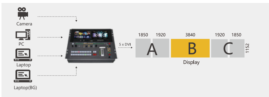
Example: Five displays, with centre "B" display using main HDMI output and window/layer
