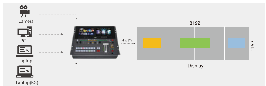
Example: Single PIPs on each of two displays as well as a PIP split across the two AUX outputs over a background
