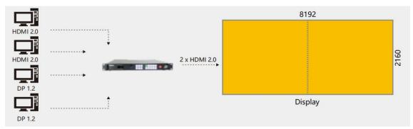
Example 1: 4K input scaled across 8K x 2K display area using two outputs, forming panoramic or wide screen display.
