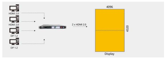
Example 2: 4K input scaled across 4K x 4K display area using two outputs, forming a seamless portrait display of high screen display.
