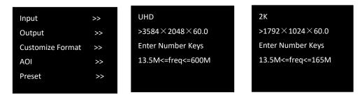
3) DVI Parameter setting and confirmation : "output >> split >>DVI splicing". Select the corresponding output outlet to set the clipping value. The clipping value (position + size) should not exceed the total output width and height of HDMI 2.0 and the clipping value of single port ≤1/2HDMI2.0 output resolution width and height.
