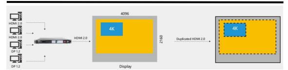
Example: 4K input scaled across a 4K output with 4K PIP source overlaid.
