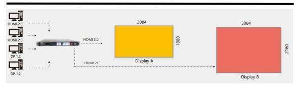
Example: Two separate inputs to two separate outputs, each at different resolution.
