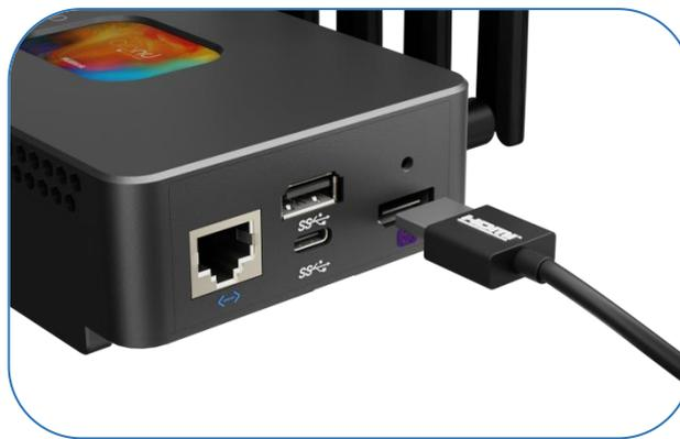
Additionally, the USB Type-A and USB Type-C ports on the bond 7UHD support UVC (USB Video Class) input. You can connect UVC-compatible device (for example, a camera) to either the USB Type-A or USB Type-C port to directly transmit video signals captured by the camera.
