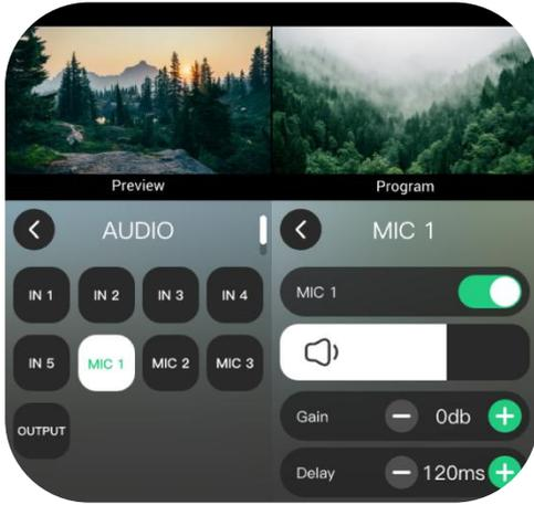
MIC 1-2 is for setting gain and delay.
