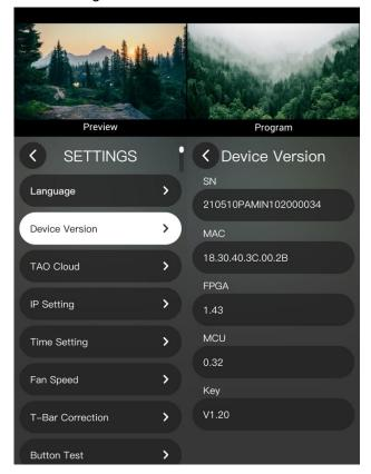
As shown in the image above, users can view the device serial number, MAC, FPGA, MCU version, and Key button version.
