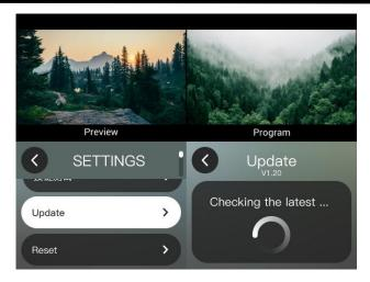
4. The system automatically checks the device's version. It displays "already the latest one" if the device is up-to-date.
