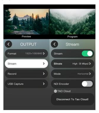
Users can adjust the bitrate and mode of the video live stream according to the actual situation. For example, if the network speed is slow, the bitrate can be switched to a lower level.
