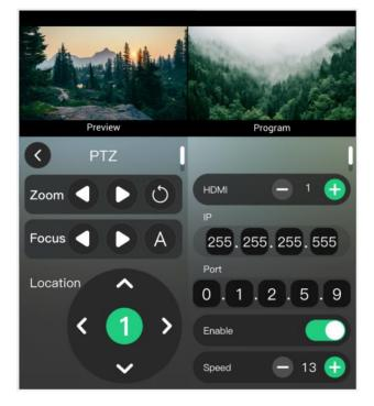
When controlling PTZ, the mini-ISO and the PTZ camera need to be in the same LAN and have the same network segment. Users can set the IP address of the mini-ISO in the "PTZ" menu. When setting the IP address, users can select different IP segments by pressing the S button and then adjust the four numbers of the IP address by the up and down buttons on the front panel. If you need to set PTZ, please select the corresponding PTZ camera signal to the PRE window by signal key 1 2 3 4 5 first.
