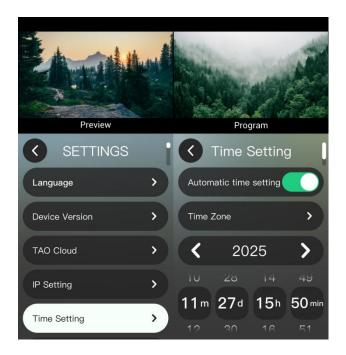
If the power-on configuration is enabled, the mini-ISO will automatically pop up this interface after power on to remind the user to set the time. After the device is turned off, the set time will be restored to the default value.
