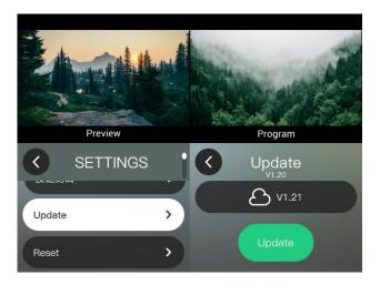
In this interface, you can press the "Update" on the right side to upgrade the mini-ISO (See <u>6.3 Upgrade Guidelines</u> for details on the steps to upgrade the device). Please make sure your network is working during the update.
