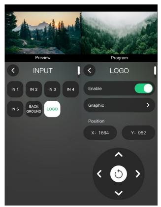
2. After selecting a LOGO, you can adjust the LOGO position using the panel on the screen. Besides, you can use the joystick to adjust the position.
