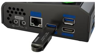
Insert the USB flash disk into the USB recording port of the mini-ISO with the RECORD silkscreen. Format your USB flash drive before using the recording function. To format the USB flash drive on the mini-ISO, proceed as follows:
