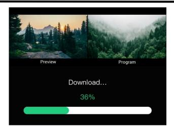
7. Please do not power off during the upgrade process. After the upgrade is completed, the device will restart automatically.
