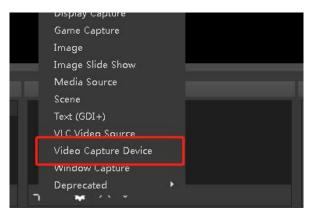
3. Choose RGBlink USB 3.0 Capture, set resolution type as "Custom" and choose Video Format YUY2. To ensure the accuracy of the output color, set the color space as "Full".
