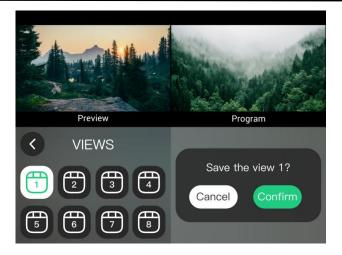
4. If you still need to modify the picture-in-picture after calling the preset, you can directly select the corresponding signal by the signal source button, and adjust the position of the screen by the joystick. All the readjusted settings will be saved in real time to ensure that you can use them directly when you turn on the computer next time.
