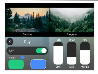
Select a color icon and adjust it. The default color is green as the background. You can touch the touch screen to select different options and slide to adjust the parameters, or use the up and down keys on the front panel of the device for fine-tuning. The default parameters of the device are: the upper limit is 1232, the lower limit 560, and the margin 602.
