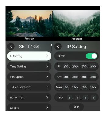
Static: If the DHCP IP distribution function is not used, users can manually set a static IP by turning off the DHCP switch.
