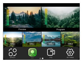
3. You can tap to turn keying on or off. The sub-screen defaults to Input 4 and the main screen defaults to Input 1.
