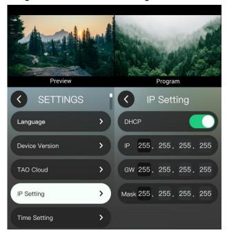
Turn on the DHCP switch to obtain an IP address automatically, and turn off the DHCP switch to configure the IP address, subnet mask and gateway manually.
