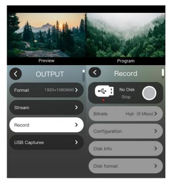
The mini-ISO will automatically recognize whether a USB flash drive is inserted or not. If no USB flash drive is inserted, the recording function can not be used.
